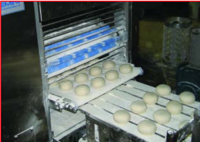
TWL and TWS divider/rounders for products with a scaling weight range of 1 ounce to 12 ounces
