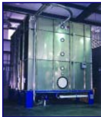
Indoor flour tanks
