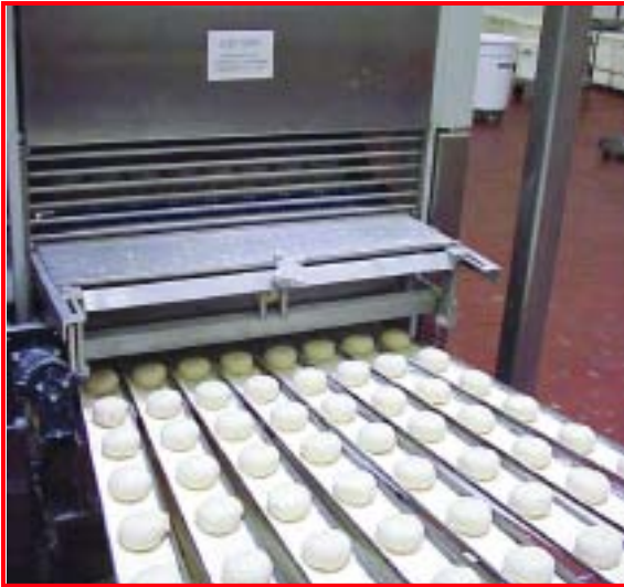
TWL and TWS divider/rounders for products with a scaling weight range of 1 ounce to 12 ounces
