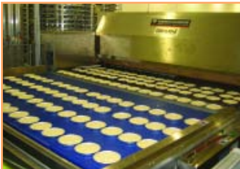
Indirect fired tunnel ovens for hearth and pan products
