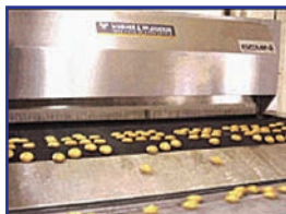
An 80-ft. indirect-fired oven was required to increase bagel baking capacity.
