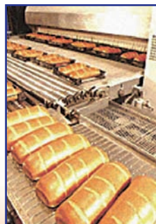
Frames assure proper shape for Ginsburg’s rye breads.
