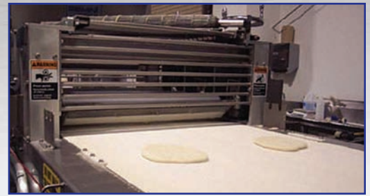
Today, 9-in. muffuletta boules run through the computerized shaping line at 70 per minute.
