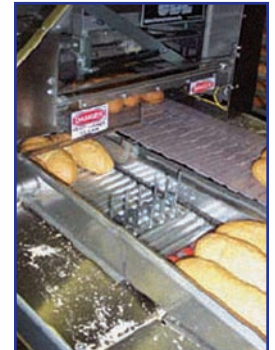
The new packaging line automatically stacks buns before bagging. A slicing system can be engaged for slicing buns when customers require.
